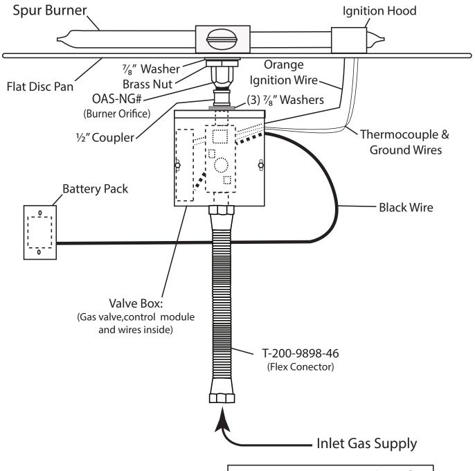
**Note**: Use joint compound or Teflon tape resistant to all gasses on all male NPT threads; not flared fittings. Ensure all connections are tight and check for gas leaks before and after assembly is complete.
