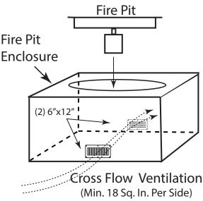
Fig 3. Cross Ventilation Example
