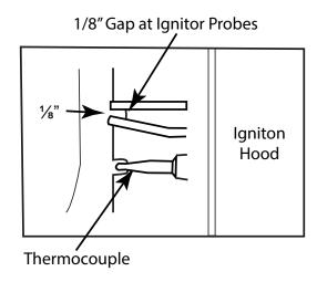
Fig. 8 Proper alignment of probes and thermocouple.
