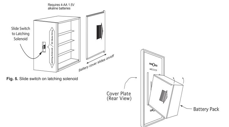
Fig. 6 Cover plate installation
