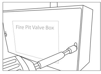
Fig. 9 Removing the cover from metal box.
