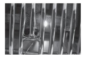
Push and turn the control knob of the burner to 'Lite". If the burner does not light in 4 seconds, turn the knob off and wait 5 minutes before attempting again.
