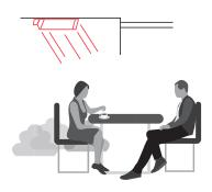
When outdoors, hang heater under protective roof or wether cover whenever possible. Even though heater is all-weather construction, it will last longer and look better if it is protected from rain and snow.
