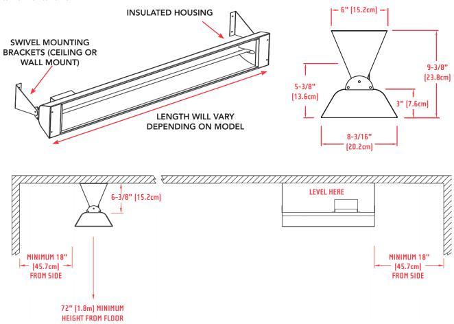
Heater must be installed with the quartz tube horizontally level. For maximum tube life, use a carpenter's level tool to find the optimum level position for the heater's body. Always maintain the minimum clearances from the heater body to any combustible materials.
