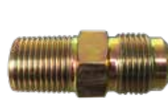
U1-8C-S (steel) 1/2" OD FLARE X 3/8" MIP (TAPPED 1/4" FIP)
