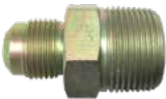
U1-8E-S (steel) 1/2" OD FLARE X 3/4" MIP (TAPPED 1/2" FIP)
