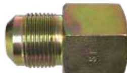
U3-10E-S (steel) 5/8" OD FLARE (15/16-16 THREAD) X 3/4" FIP
