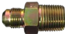
U1-6D-S (steel) 3/8" OD FLARE X 1/2" MIP (TAPPED 3/8" FIP)
