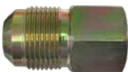
U3-10D-S (steel) 5/8" OD FLARE (15/16-16 THREAD) X 1/2" FIP
