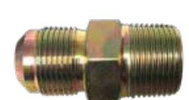
U1-10E-S (steel) 5/8" OD FLARE (15/16- 16 THREAD) X 3/4" MIP (TAPPED 1/2" FIP)
