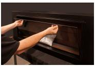
Carefully remove glass panel by pulling on the tabs located on the left and right side of the firebox.
