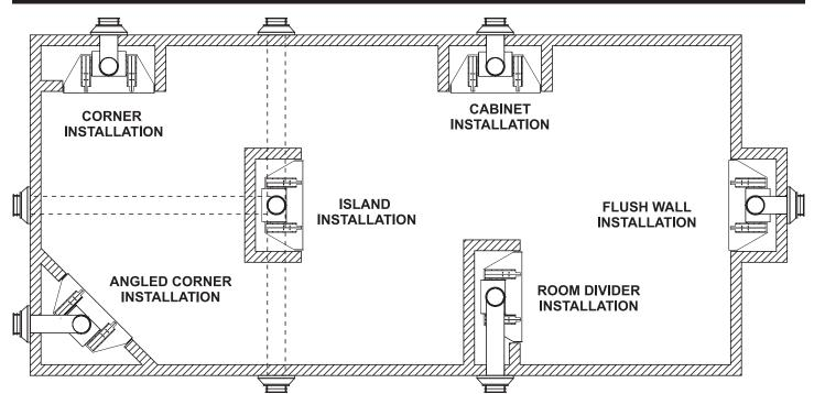
**NOTICE**: Island and room divider installation are possible as long as the horizontal portion of the vent system does not exceed 20 feet with a minimum vertical run of 8 feet. Refer to Venting Section (pages 16 - 27).
