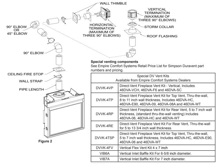
NOTICE: Additional pipe may be required for proper venting.
