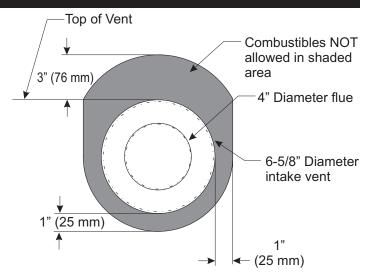
Figure 23 - Hard Pipe Vent Clearance
