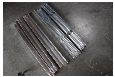
The top of the firepit is made up 8 pieces of 48" track/Stud. There are 2 sets of each of tracking.
