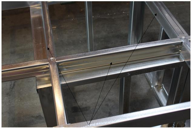
Place the top onto the base and screw from the rails of the top into the base to hold the top on. Place approx. 3 screws on each side.
